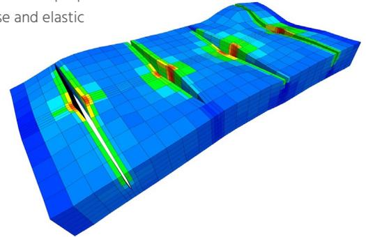
Design and optimize well completions by visualizing hydraulic fracture initiation and propagation using discrete finite elements.
