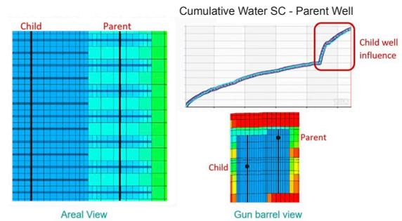
Figure 2: Overlapping fractures and parent well water production
