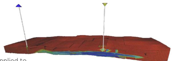
3D view of fine grid simulation model, showing the property  $N_2Cl$  mole fraction. Injected water has a lower salinity than formation water
