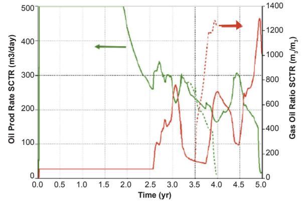
Comparison of oil production rates (green lines) and GOR (red lines) for foam case (solid lines) and no foam case (dashed lines)
