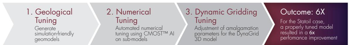
The workflow was applied to a geologically complex, highly heterogeneous 24-well pair SAGD project, located in Alberta, Canada. The model has over 2.52 million active gridblocks and simulated ten-years of production forecast. The application of this workflow improved numerical stability and the run-time of multi-pad SAGD simulation models. Some of the workflow recommendations are specific to thermal processes; however the principles are generally applicable to other types of reservoirs.
