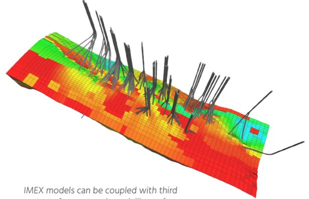
IMEX models can be coupled with third party surface network modelling software for simultaneous modelling of both the reservoir and surface network.
